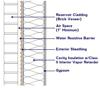
Figure 3: Insulated wall assembly w/brick veneer
