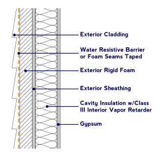
Figure 5: Wall assembly w/exterior rigid foam
