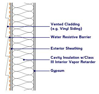
Figure 2: Insulated wall assembly w/vented cladding
