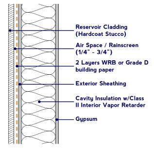
Figure 4: Insulated wall assembly w/exterior plaster
